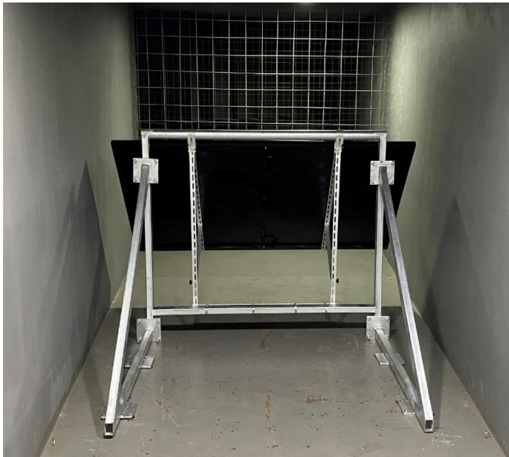
Figure 3. PV module back side facing wind (180°)
